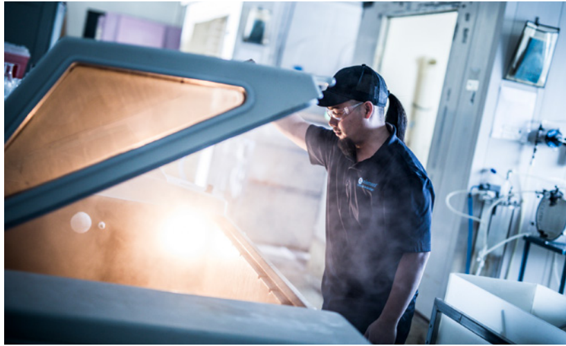
A salt spray test (also called salt fog testing) uses high-saline environments to measure the corrosion resistance of products, paints, and coatings over extended periods.
